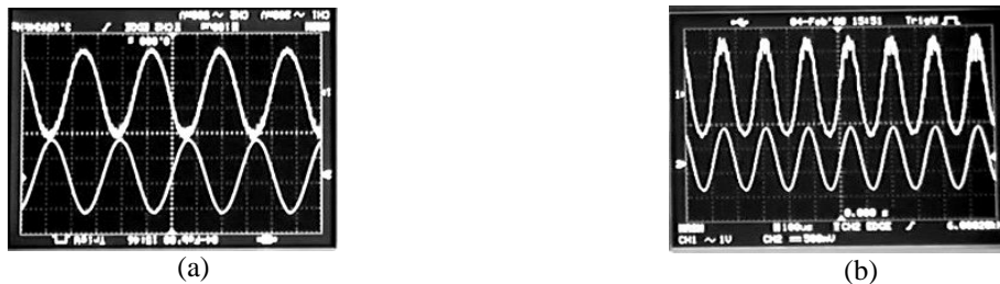
Fig. 4. Snapshots of oscilloscope traces which demonstrate an operation of two-channel adaptive measurement system: first channel (a), second channel (b). Trace on a top is a detected signal, while bottom trace represents a modulation signal which excites vibration with amplitude of 10 nm.
